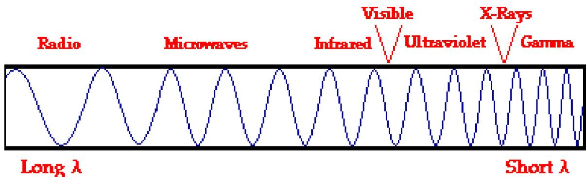
Since EM radiation travels as a wave, we can describe it in terms of wavelength ( $\lambda$ ), frequency ( $f$ ) or energy ( $E$ ).
